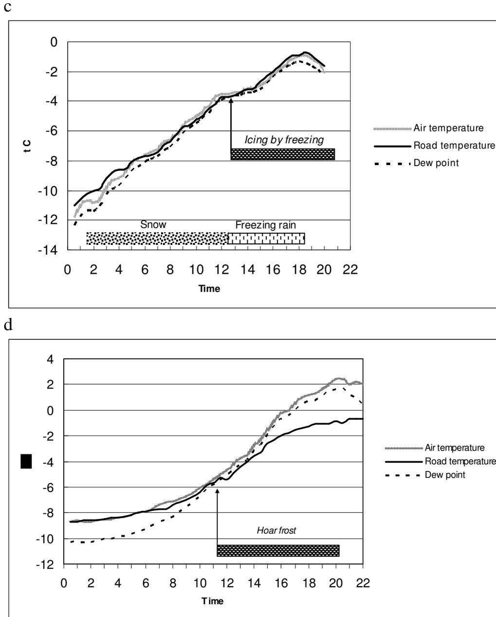
Fig. 1 c, d. Model graphs of the variation of parameters for basic types of ice: freezing rain (c), frost (d)
