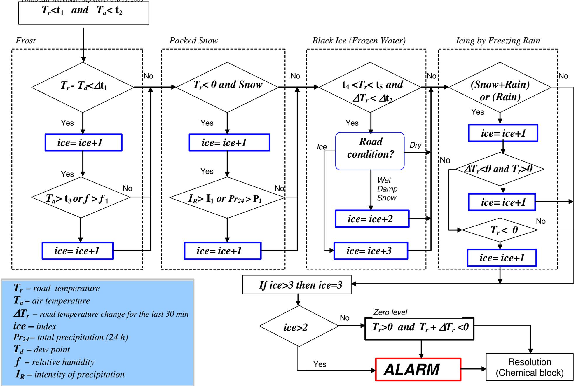
Fig. 2. The block of situation diagnosis consists of four modules: Frost, Packed Snow, "Black Ice" (Frozen Water), Icing by Freezing Rain
